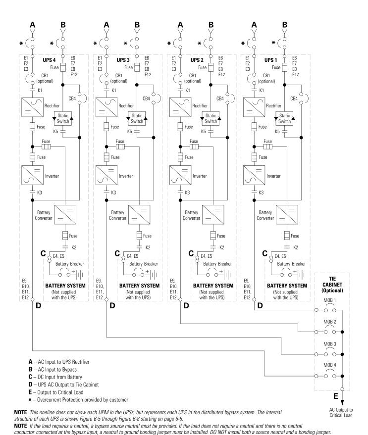
Figure 6-23. Typical Distributed Bypass System (3+1 and 4+0 Configurations)
